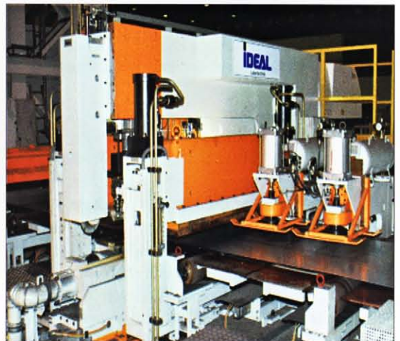
ⓐ Fig 10 LAS 300 cutting/welding machine
