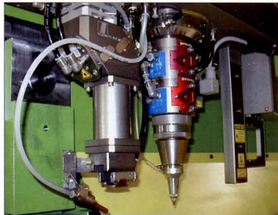
Fig 2 Laser cutting/welding head and plasma control
