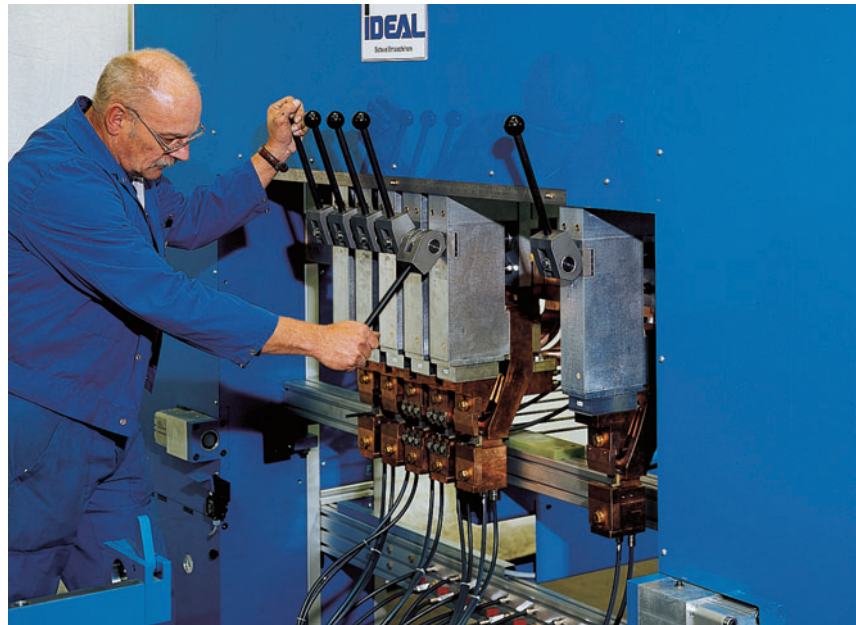
Setting of welding heads to line wire pitch
