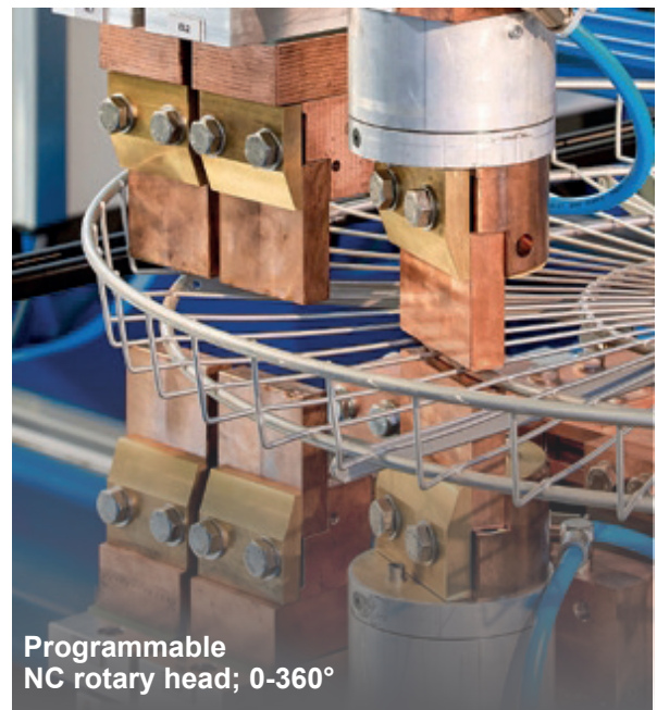
Welding gun and rotary electrode enable a larger product portfolio
